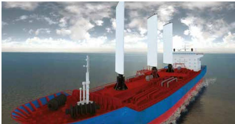
of traditional sails and existing novel designs. The system is suitable for a wide range of vessels: from fishing and recreational vessels to large merchant vessels. Their key solution is completed with a user friendly automated control system and a route optimization software which brings
